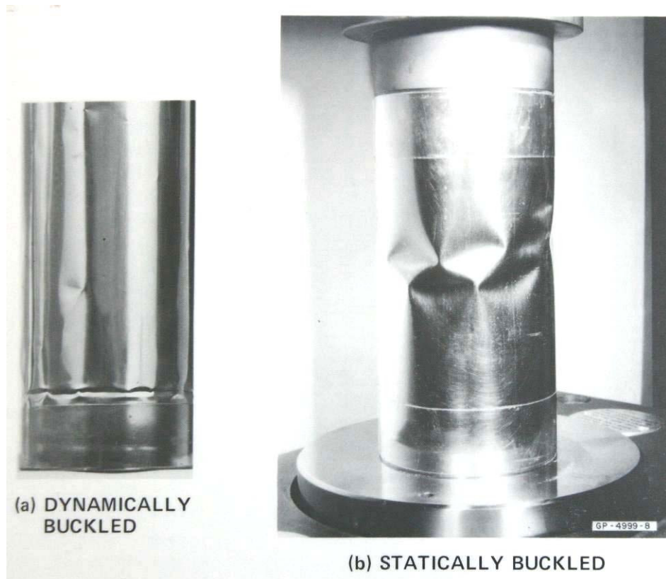
Figure 1.4: Comparison of dynamic and static post-buckled patterns.
